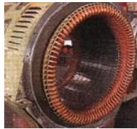
Primary Stator Rewind
